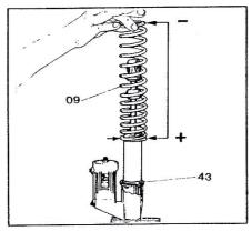
Assemble spring (09) making sure that the wider part always touches the spring adjuster (43). This is not the case when biconical springs are mounted.
