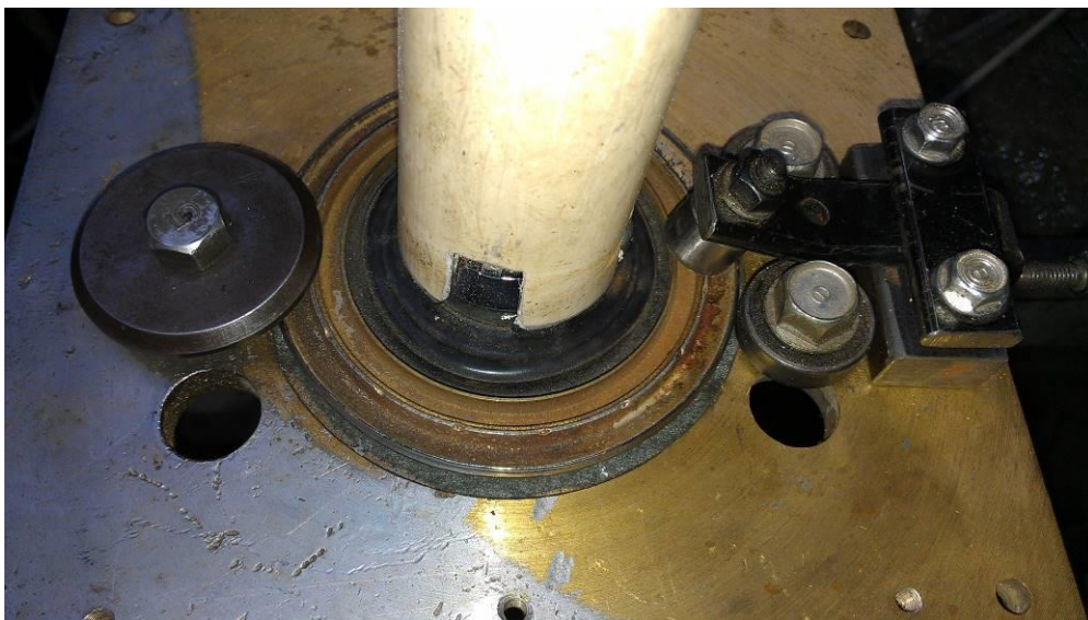
Here the 'un-rolling' bearing and arm are fitted in place. The white PVC tube as the handle for turning the tank cap
