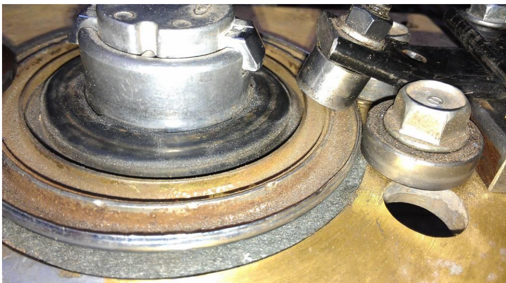
Here the rolled edge and the action of the angled bearing is clearly visible.
