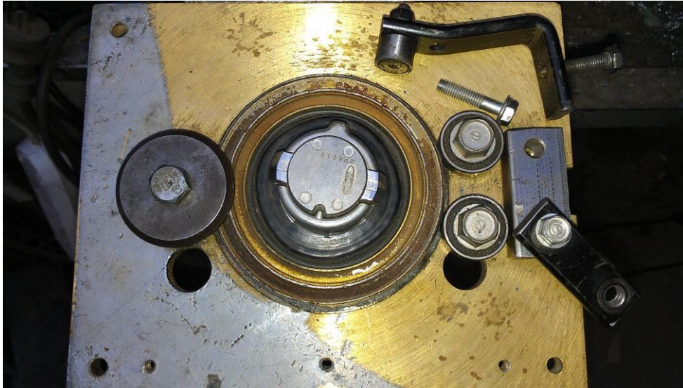
Tank cap slipped under the washer on the left and dropped against the guide rollers at the right
